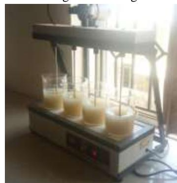
Fig.4: Jar test apparatus
