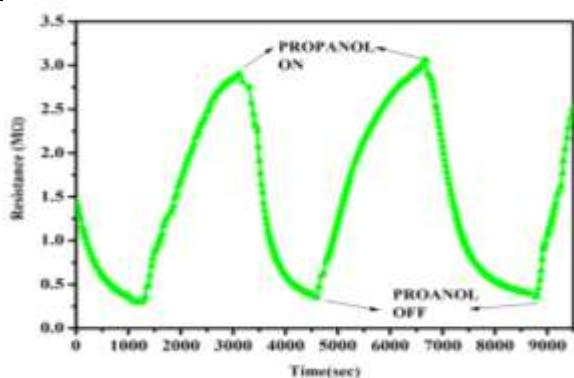
Fig.3b: Repetitive resistance response of propanol
