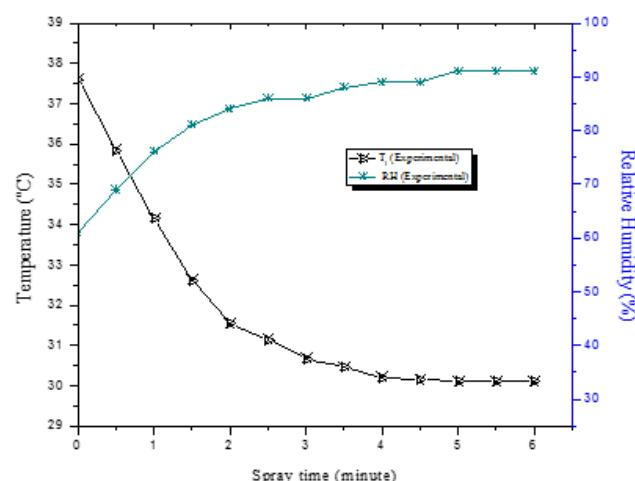
Fig. 4: Temperature and RH profiles with continuous fogging
