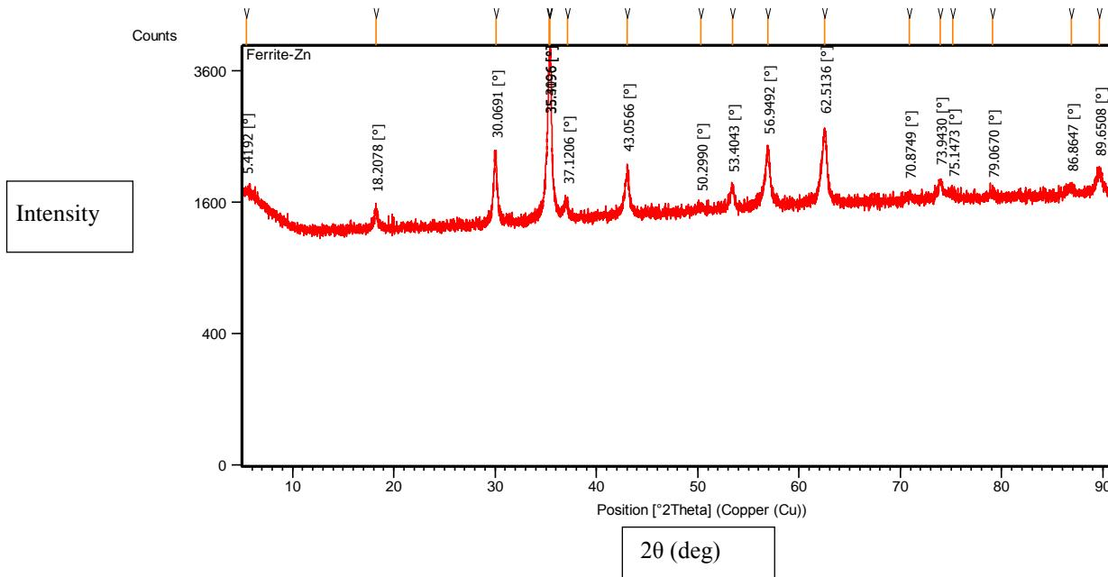
Fig.1: XRD Pattern of Nano-Composite  $Ni_{0.5} Cu_{0.2} Zn_{0.3} Fe_2 O_4$
