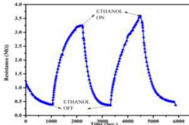
Fig.3a: Repetitive resistance response of ethanol
