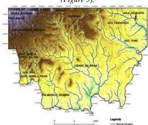
Fig.3: Draining network generated from a DTM.
