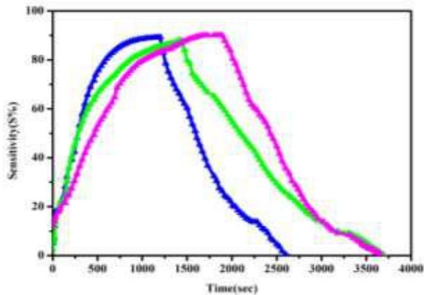
Fig.4: Sensitivity of NZF towards ethanol (blue), propanol (green) and butanol (pink) at room temperature.
