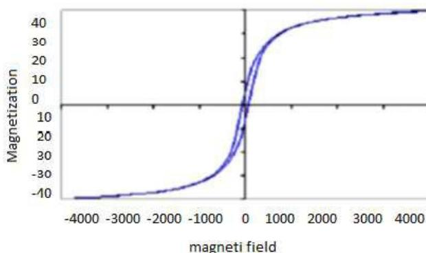
Fig.4: Magnetic hysteresis loops for  $Ni_{0.5} Cu_{0.2} Zn_{0.3} Fe_2 O_4$
