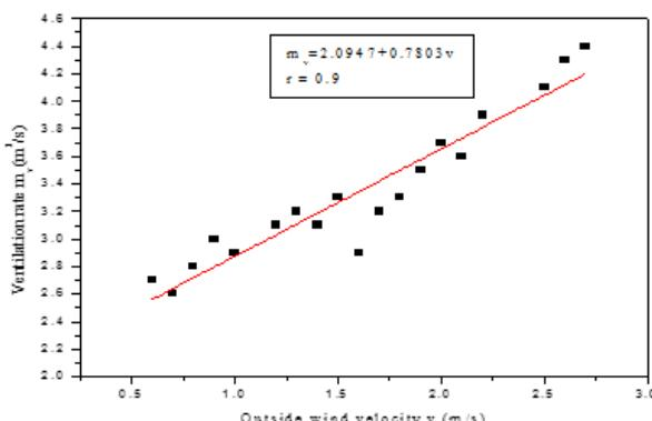
Fig. 3: Variation of ventilation rates against wind velocity
