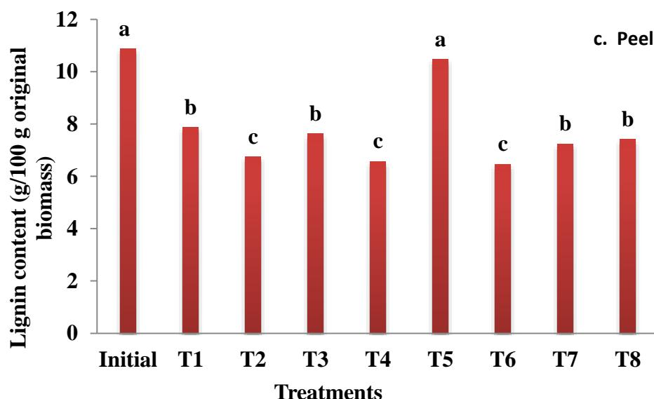
Fig.1 (a-c): Lignin changes in MW-irradiated or steam-exposed biomass subjected to AHP treatment; bars with different alphabets are significant at  $p < 0.05$ .
